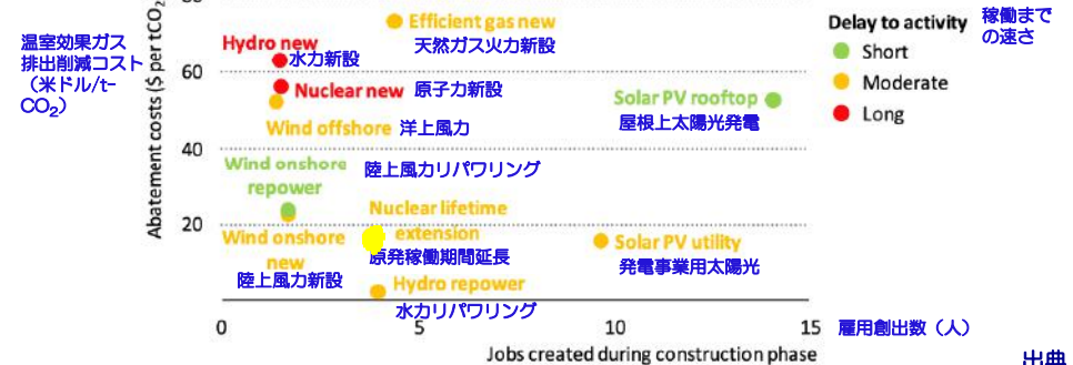
Figure 2.3 Job creation per million dollars of capital investment in power generation technologies and average CO 2 abatement costs
